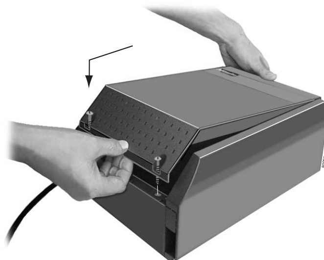
Figure 8: Replacing the DS2000 Cover
